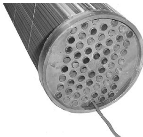
Clean Aftercooler Core
