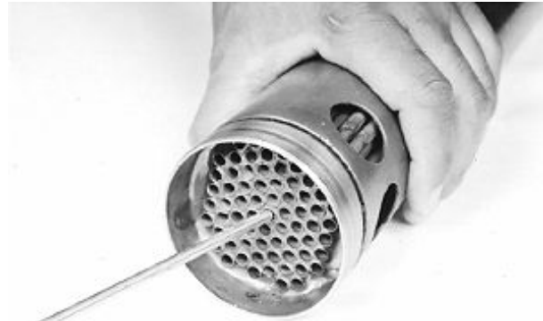
Clean Heat Exchanger
