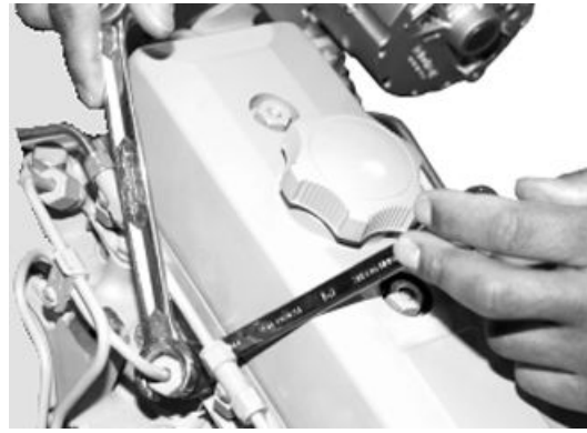
Loosen Fuel Pressure Line
