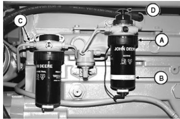
Bleed Fuel System
