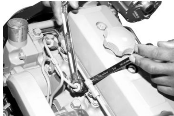
Bleed At Fuel Injection Nozzles
