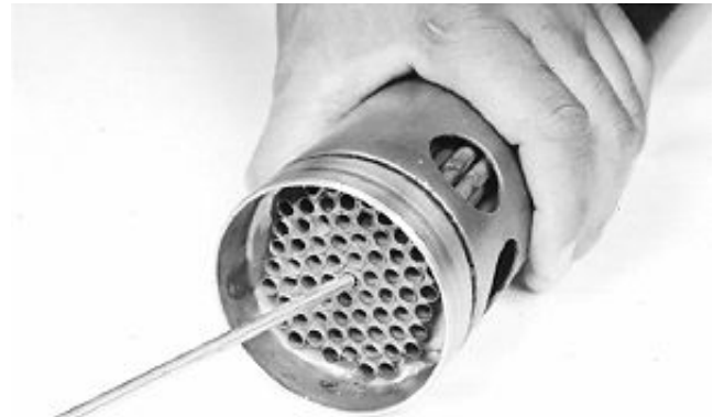
Clean Heat Exchanger
