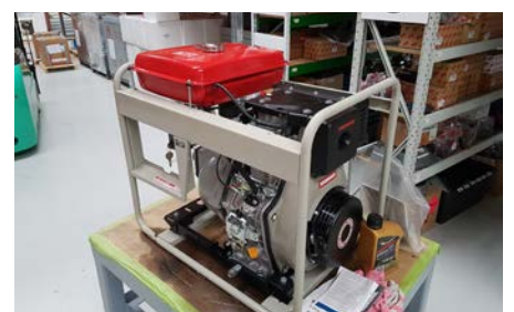
Yanmar L100N (10hp) powered pump
