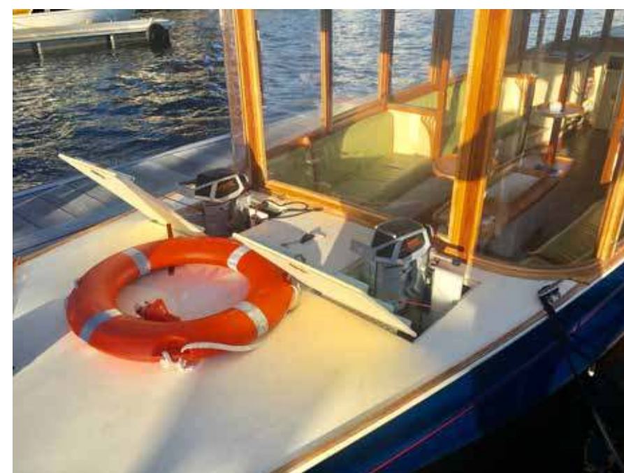
Torqueedo Cruise 4.0 provides all the power the Little Ferry needs
