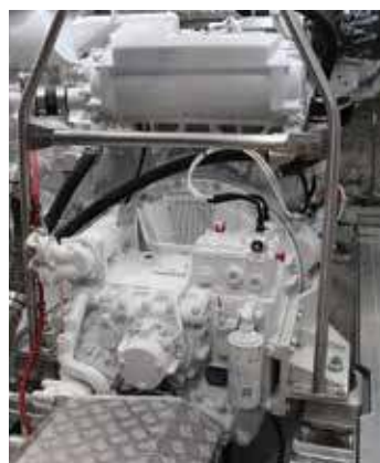
The Yanmar 6AYM-WGT in the engine room
