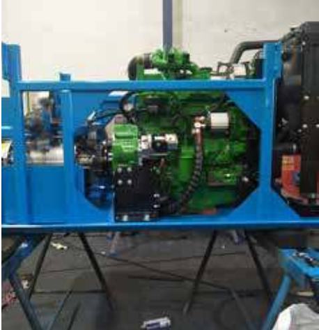
The John Deere 4045T2 was being installed on the Tefco trailer
