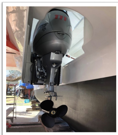
The outboards are mounted on a jacking plate, so they can be jacked up before being tilted when sailing.
