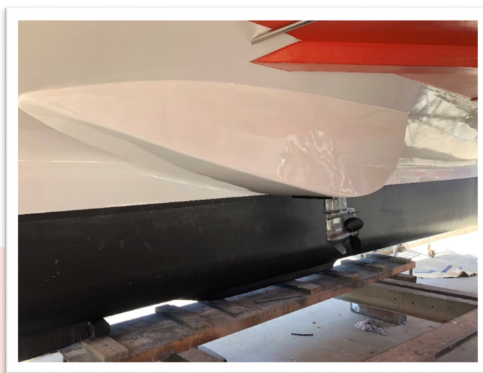
The outboards are mounted on a jacking plate, so they can be jacked up before being tilted when sailing.
