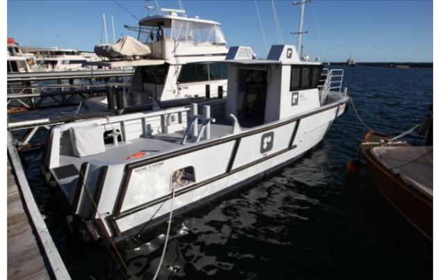
Powered by a pair of Yanmar 6LYA 370 mhp diesel engines, the Go Centaur is a distinctive vessel. Destined for use at Port Hedland and operated by Go Marine, this is a tough workhorse. From any angle the hull has the lines of a rugged commercial vessel - high freeboard, small cabin, huge work deck and heavy duty tow post.
