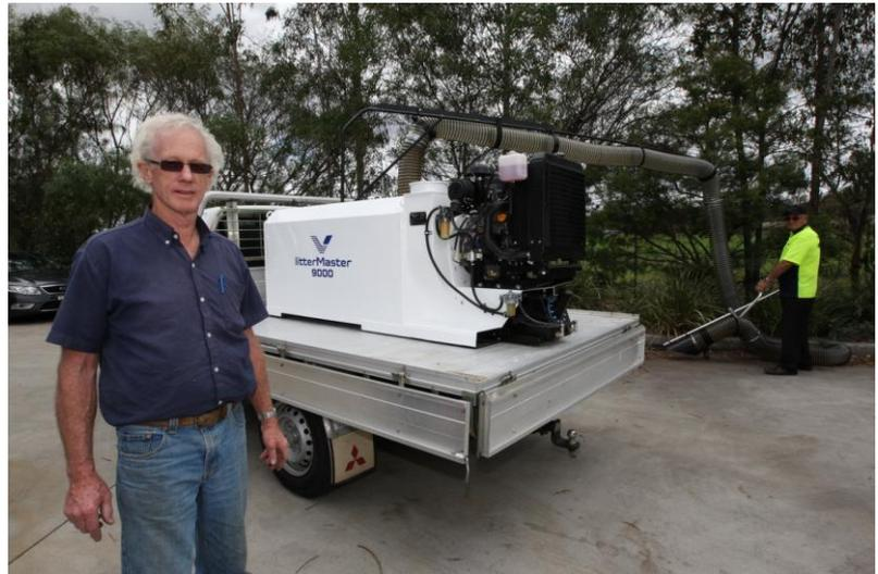
The demand for this particular unit, the Litter Master 9000, came from a group of local Councils looking for collection equipment which could be used in the field. The technical specification called for a vacuum unit which could be carried on a conventional drop sided ute, be operated by a two man crew and be used by workers in parks and gardens to keep public spaces clean of litter, such as litter and broken glass, and seasonal garden green waste.
