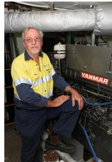
Fodico Marine Group is currently constructing the 'Pacific Titan', a new-build 26m 30T BP shallow draft utility tug due for delivery early 2016. The 'Pacific Titan' has been specified with a full complement of five Yanmar marine diesel engines, including main engines (2 x 6EY17W) and gearboxes, generators (2 x 6CHL-TN), and hydraulic power unit (1 x 6HA2M-WHT).
