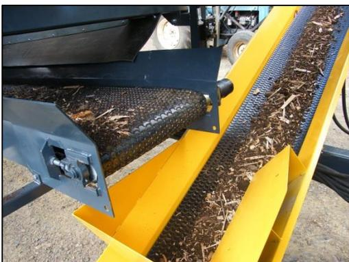
**Photograph D:** *Waste material is neatly discharged along the waste conveyor into a skip*
