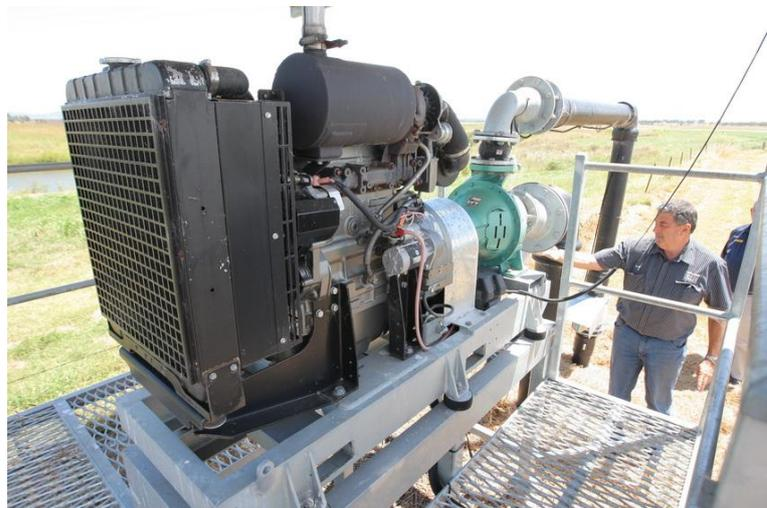
To compound matters, periodic flooding at the pumping station is an annual event. To protect the pumping station from flood damage, local Yanmar Dealer Bob Dover of Dover and Sons, constructed a sturdy elevated platform from galvanised steel.
