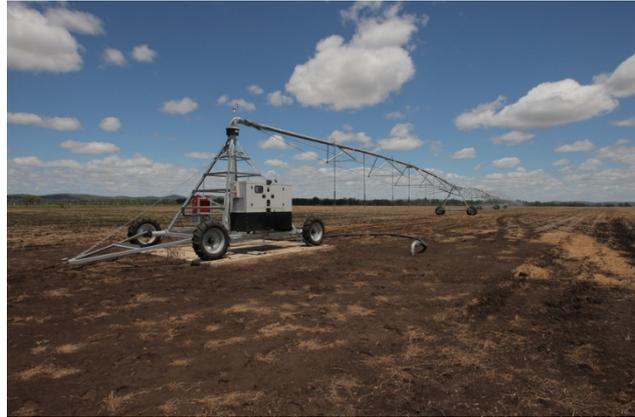
Mounted to the frame of the Zimmatic unit is a purpose built Yanmar Centre Pivot Generator (CPG) pack. This is supplied as a complete turn-key system by the Australian Yanmar Distributor, Power Equipment.
