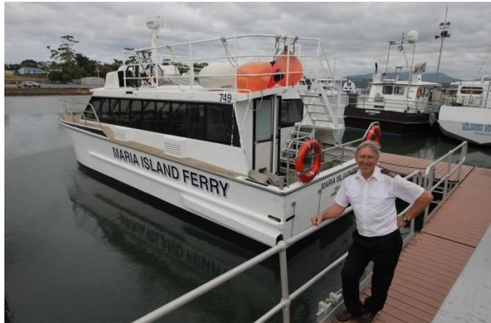
As a direct result of the Yanmar re-power, the steaming time from Triabunna to Maria Island has been reduced by 8 minutes, each way. Fuel consumption has also been reduced by 30%.
