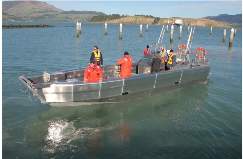
The Rapid Response Vessel has a drop down boarding ladder mounted at the bow and the hull has been designed so that people can also be pulled over the side.
