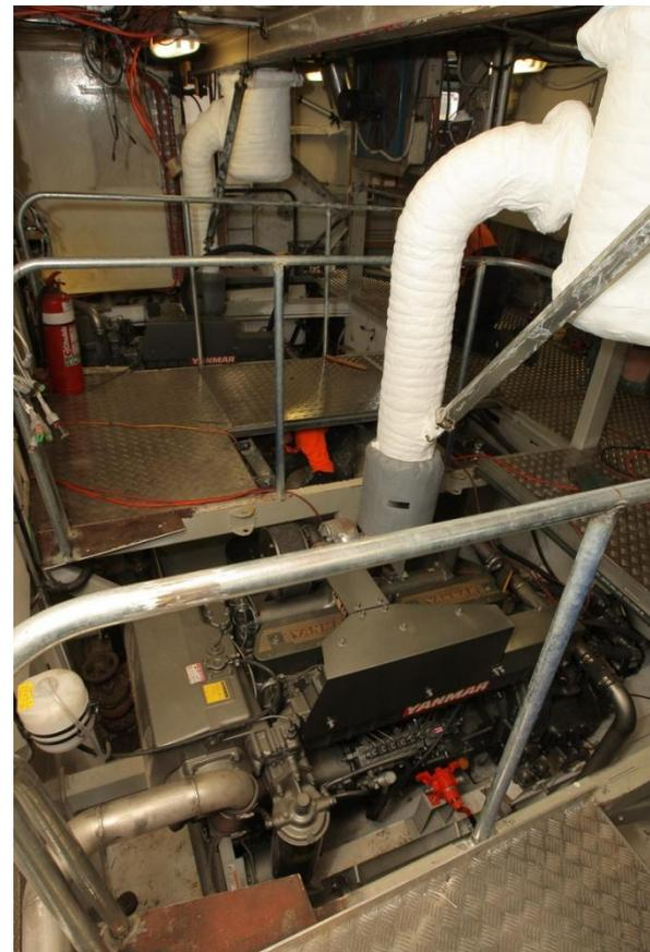
The Yanmar 6HA2-WHT model is an in-line six cylinder marine diesel engine that displaces 13.14 litres and weighs 1340 kgs without the gearbox. Maximum power output is 350 mhp (257 kW) at 1950 rpm with an alternative rating of 278 mhp (204kW) also offered.
