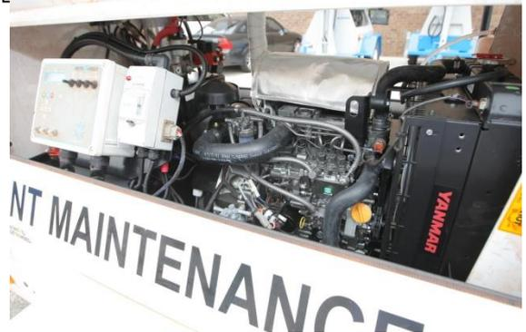
*Above: In with the new – a fresh Yanmar 3TNV70 fitted to the BHP lighting tower built by Briteforce.*
