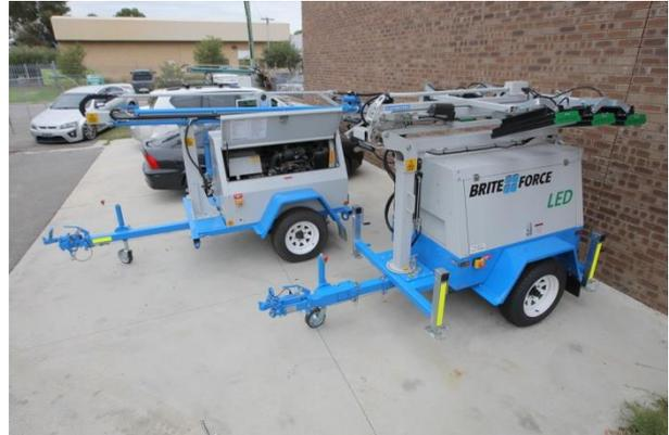
*Above: The two models of lighting tower on offer from Briteforce, both Yanmar 3TNV70 powered and both with LED heads.*
