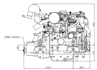
3YM30AE with KM2P-1 marine gear (Not to be used for engine installation)
