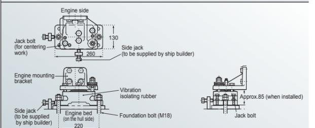
Note: Specially arranged engine mounting bracket is to be used.
