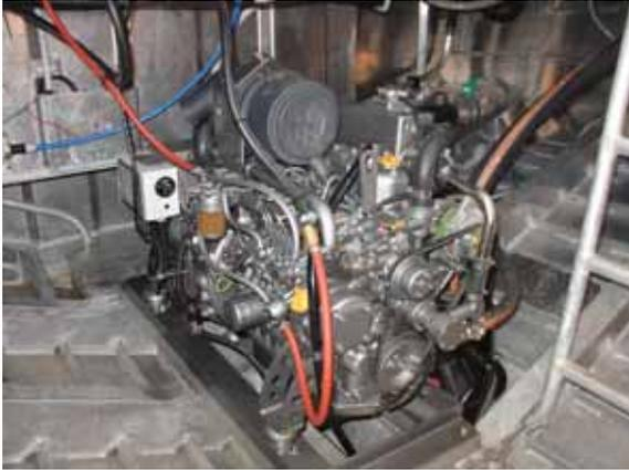
engine oil sump pump. The Gen-Set has been installed using a Foreshore Exhaust custom built & supplied exhaust system, utilising both a waterlock muffler and gas separator type muffler, thus offering both added protection against water running back into the exhaust whilst the Gen-Set is switched off and the vessel is operating in heavy sea conditions as well as a much quieter operation.
