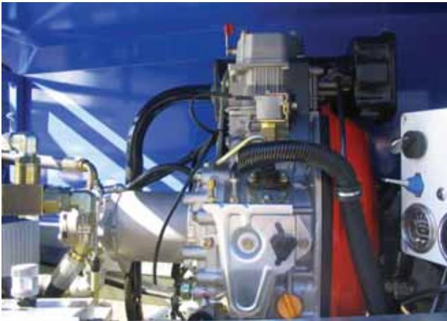
For several years now Upton Irrigation of Toowoomba Queensland have been using the Yanmar model L70AE-DE single cylinder Air Cooled Diesel engine to power their "Boom Irrigator".
