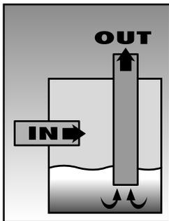
Fig. 2: How a water-lift muffler (top) works.
